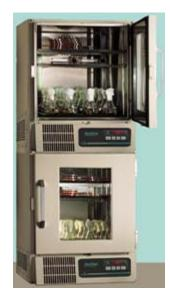
Two Innova 4200/4230 shakers can be stacked using the optional stacking kit.
